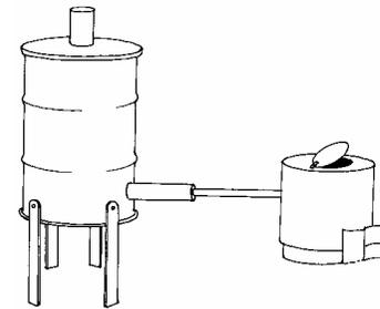
Fig. 12.2. Modified drum kiln
