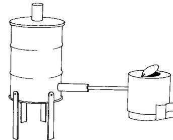
Fig. 12.2. Modified drum kiln
