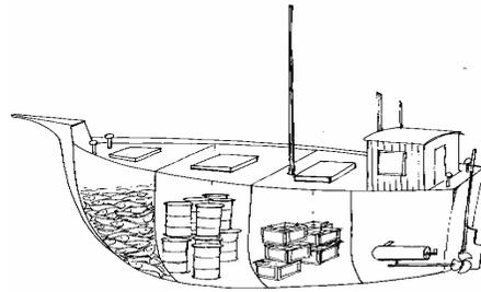
Fish is ice-stored on board vessel by 3 methods:
