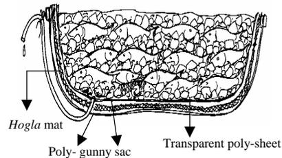
Place an adequate size of mat of plant leaves, *Hogla* in side the basket (on the 1<sup>st</sup> layer of gunny sac) to cover the whole area inside. Put another layer of equal size polythene gunny sac on *Hogla* layer and stitch these 3 layers of wrapping materials (1 layer *Hogla* in between 2 layers of gunny sac) with nylon twine to the basket so that all wrapping materials remain fixed with the basket.
