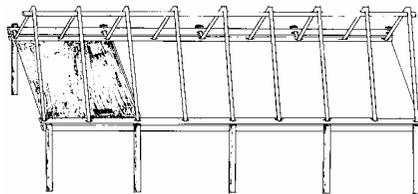
On top of one end of the platform, a galvanized iron sheet, painted black, is laid. In the case of the 20-foot long platform, this covers 4 feet of the surface. This black surface
