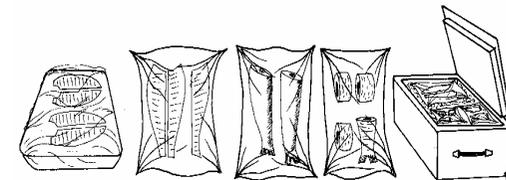
Materials used for modified atmosphere packing must be completely impermeable to gases in order to maintain appropriate gas mixture in the pack. Vacuum packaging is also done that requires high gas protective packaging film like polyvinylidene chloride or polyester.
