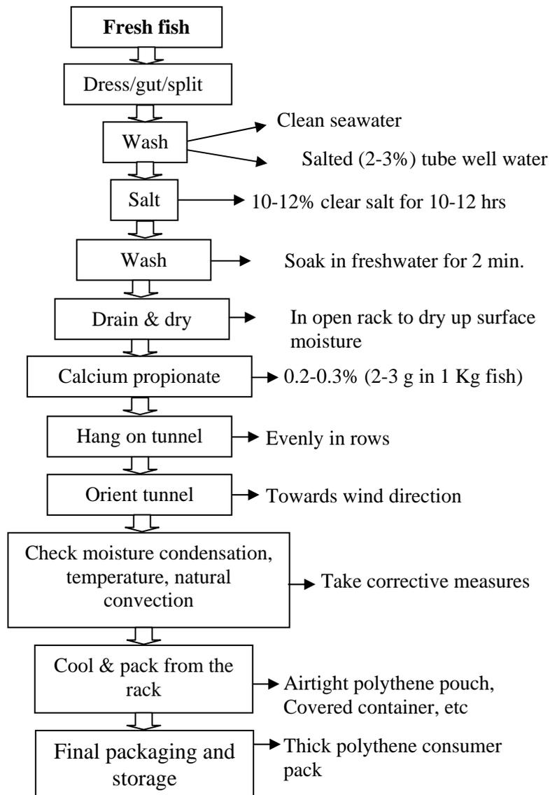
Fig. 11.4. Scheme for the drying of fish in solar dryer
