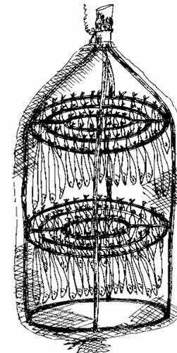
effective in drying Bombay duck, ribbon fish, carp, pomfret, jewfish, etc. in both house-hold and small-scale commercial operations.
